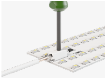
Easy conductor removal, e.g., via operating tool (Item No. 206-859) or "twist & pull" (max. 10 x, no re-connection of smaller conductors possible)
