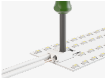
Insert/remove fine-stranded conductors by lightly pressing on push-button, e.g., via optional operating tool (Item No. 206-860).
