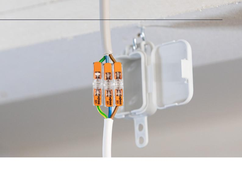
bution boxes in industrial applications. Two variants of the inline splicing connector are available, both with EN and UL approvals: one version has a transparent cover for conductor cross-sections from 0.2 to 4 mm² (stranded only up to 2.5 mm²) for all standard applications. The other version uses a white cover (favored in North America) for the extended connection range with AWG-12 conductors.
